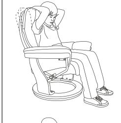
To Adjust Headrest: Place both hands over shoulder as shown in diagram. Gently pull with both hands to desired position.
