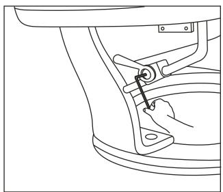
To adjust tension on glide action. With 4mm Allen Key adjust clockwise to tighten grip and anti clockwise to loosen. Note do not over tighten as handle will not lock properly.
