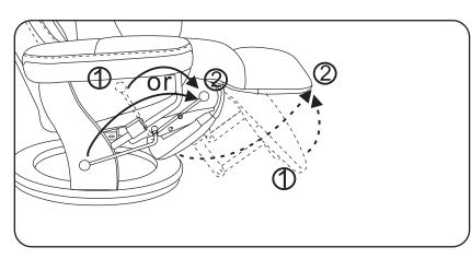
Push lever forward to position @ or push lever forward straight to position @ from down position
