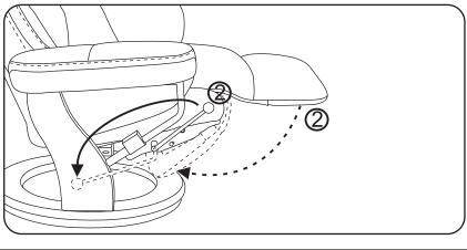
To stow lift from position ② pull lever back to down position
